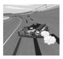
Oversteer: In NASCAR circles, the word "Loose" is more commonly used to refer to oversteer. A loose car's rear tires lose grip with the pavement sooner than the front wheels do, when the car is traveling around corners at high speed. The car begins to "fishtail" as the rear end swings toward the outside. This is caused by a lack of weight or downforce at the rear end.
