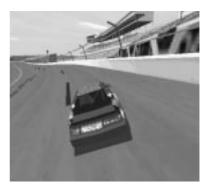
Understeer: You're more likely to hear the words "Pushing" or "Tight" used to describe understeer. A car that is pushing will lose grip with the pavement at the front wheels, before the rear wheels lose traction. This causes the car to drift out near the wall in corners, and feel like it won't turn sharp enough in general. This can be caused by a lack of weight or downforce at the front end.
